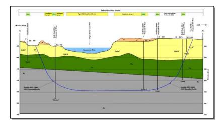
engineering geological services to characterize the type and engineering properties of soil and rock materials that would be encountered during the twin 1,800-lineal-foot HDD crossings. Our services included onshore and overwater geophysical surveys, an extensive drilling and sampling program, deep test pits to observe cobble and boulder dimensions, and an elaborate geotechnical laboratory testing program. Using those data, we
