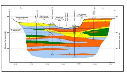
used to install up to about an 18-inch diameter water pipeline. Methods evaluated included microtunneling, pipe ramming, horizontal directional drilling, jack-and-bore, and pipe jacking.
