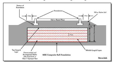
District did not have sufficient budget for construction of deep foundations. CGi evaluated and recommended the use of a geogrid reinforced composite raft embankment beneath the structure, which is both economical and relatively easy to construct. Based upon our recommendations, the project was reviewed by California Geological Survey and approved by the California Division of the State Architect without comment.
