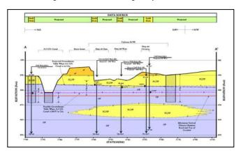
conditions that would be encountered during construction. Based on those services, CGI developed geotechnical design and construction recommendations for the installation of the pipeline. The pipeline was successfully rammed in place in April 2009, making it one of the longest pipe ramming reaches completed for this class of pipeline to date.
